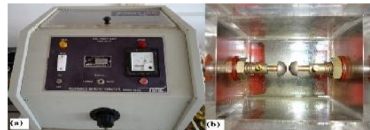
Fig. 2. (a) Oil Breakdown Voltage Test Kit (front view), (b) Internal view of oil container and electrode.
