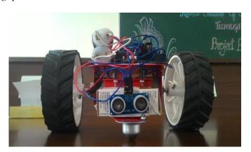
Here we are using arduino microcontroller with bluetooth module and ultrasonic sensor to make automatic and mobile controllable robot. We had coded the robotwhich will work with its own control
