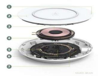
The main wireless standard is Qi (pronounced as "Chee"). Qi is a standard that has been developed by the Wireless Power Consortium (WPC) for inductive charging over distances of up to 40mm. Qi chargers has been adopted by many companies. But the energy consumption of the wireless charging is 50% higher than the wired charging.
