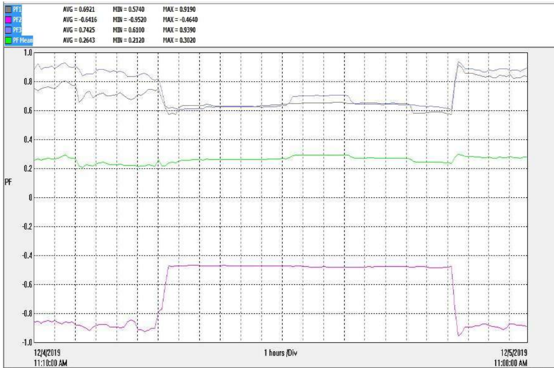
Fig.69 Shows the power factor (PF) for 24 hours from 4/12/2019 11.00AM to 5/12/2019 11.00PM Inference: unbalance found in Phase 2. Need to improve PF.
