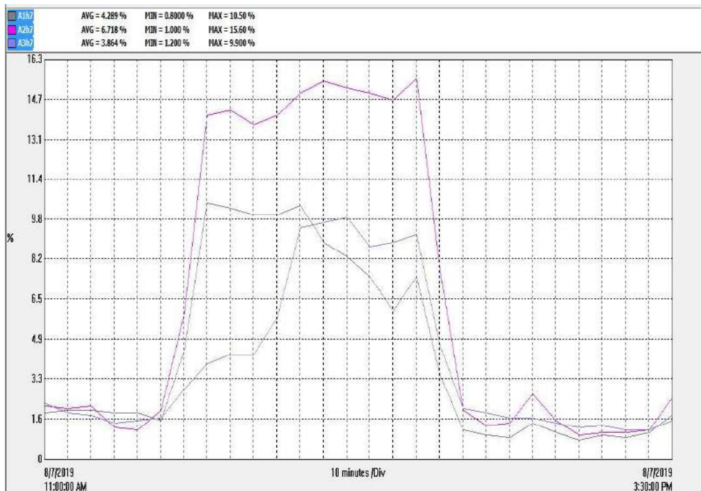
Fig.32 Shows the 7 th order THD (voltage harmonics) for 4.30 hours from 7/8/2019 11.00AM to 7/8/2019 3.30PM Inference: Harmonics seems to be normal. No need of harmonic filters.
