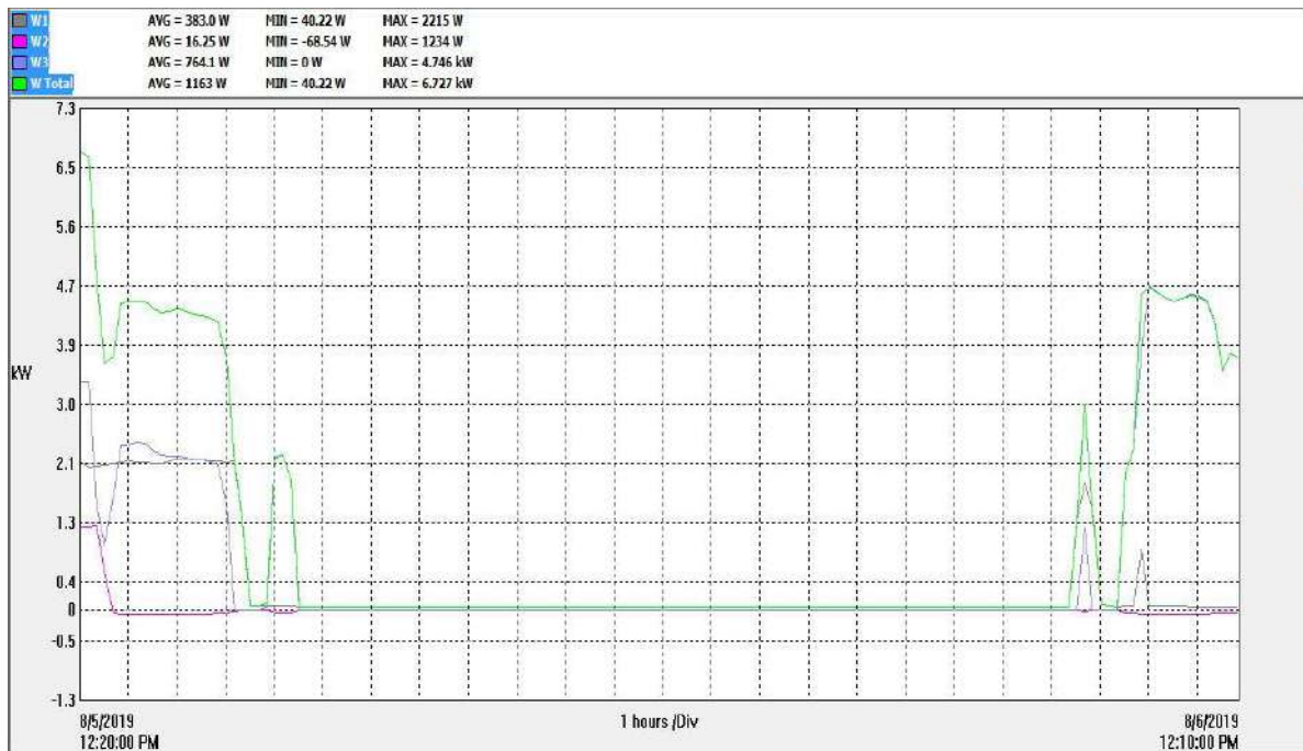
Fig.9 Shows the power (kW) for 24 hours from 5/8/2019 12.20PM to 6/8/2019 12.10PM Inference: power distribution is not balanced. Phase 2 is found to be unbalanced and it loaded only 2% of the total.
