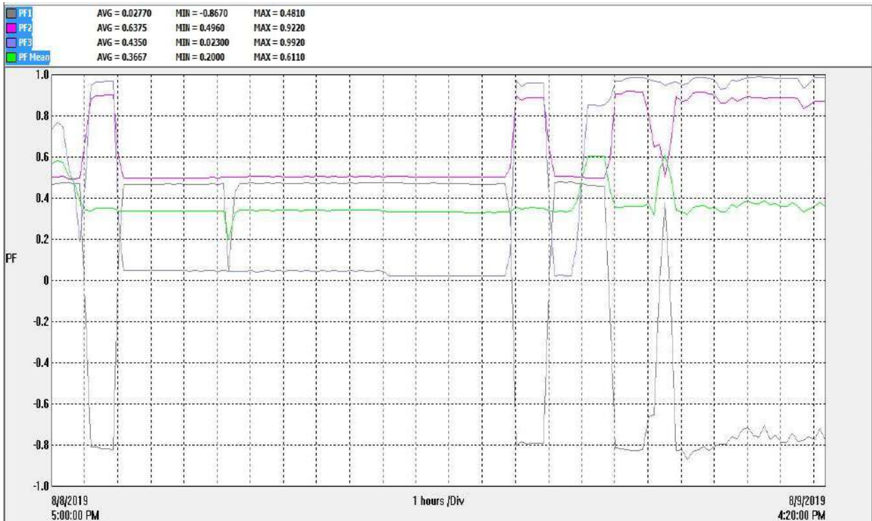
Fig.45 Shows the power factor (PF) for 24 hours from 8/8/2019 5.00PM to 9/8/2019 4.20PM Inference: Unbalanced found here. Need to be improve the PF.
