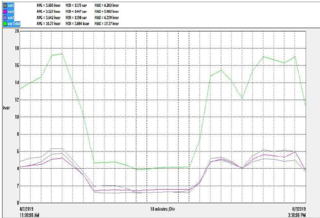
Fig.29 Shows the reactive power (kVAR) for 4.30 hours from 7/8/2019 11.00AM to 7/8/2019 3.30PM Inference: KVAR shows normal condition.
