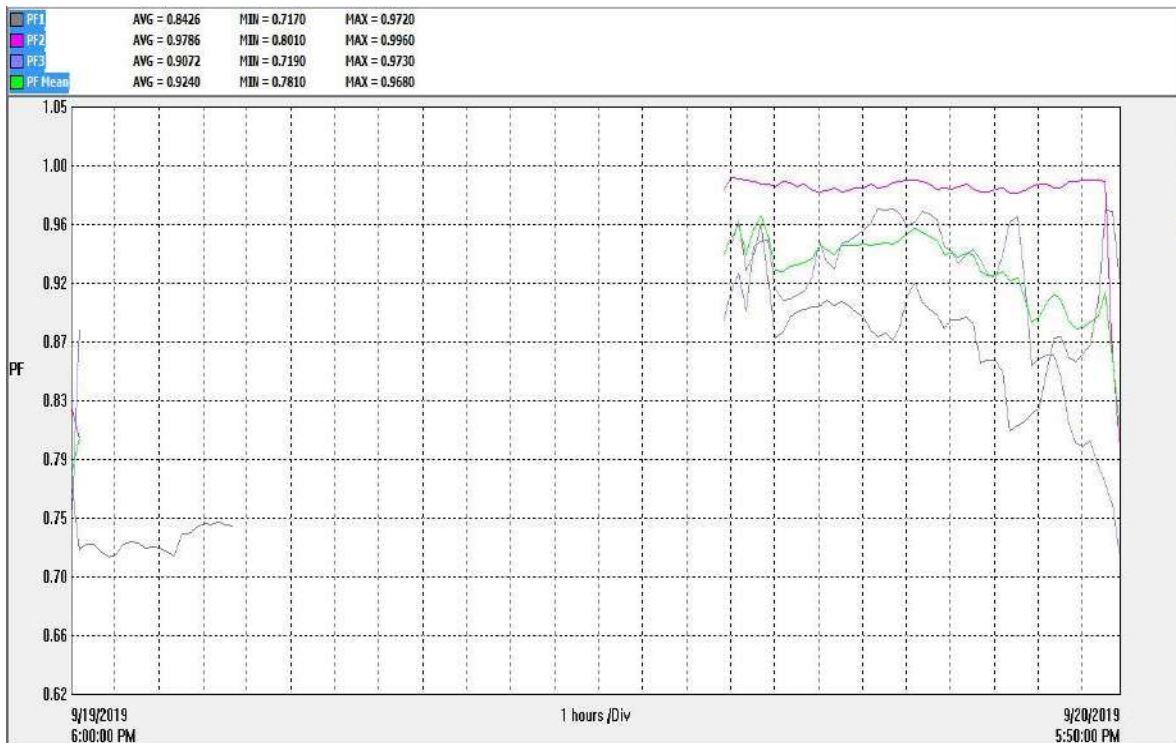
Fig.109 Shows the power factor (PF) for 24 hours from 19/9/2019 6.00PM to 20/9/2019 5.50PM Inference: No unbalanced found here. Need to improve the PF.
