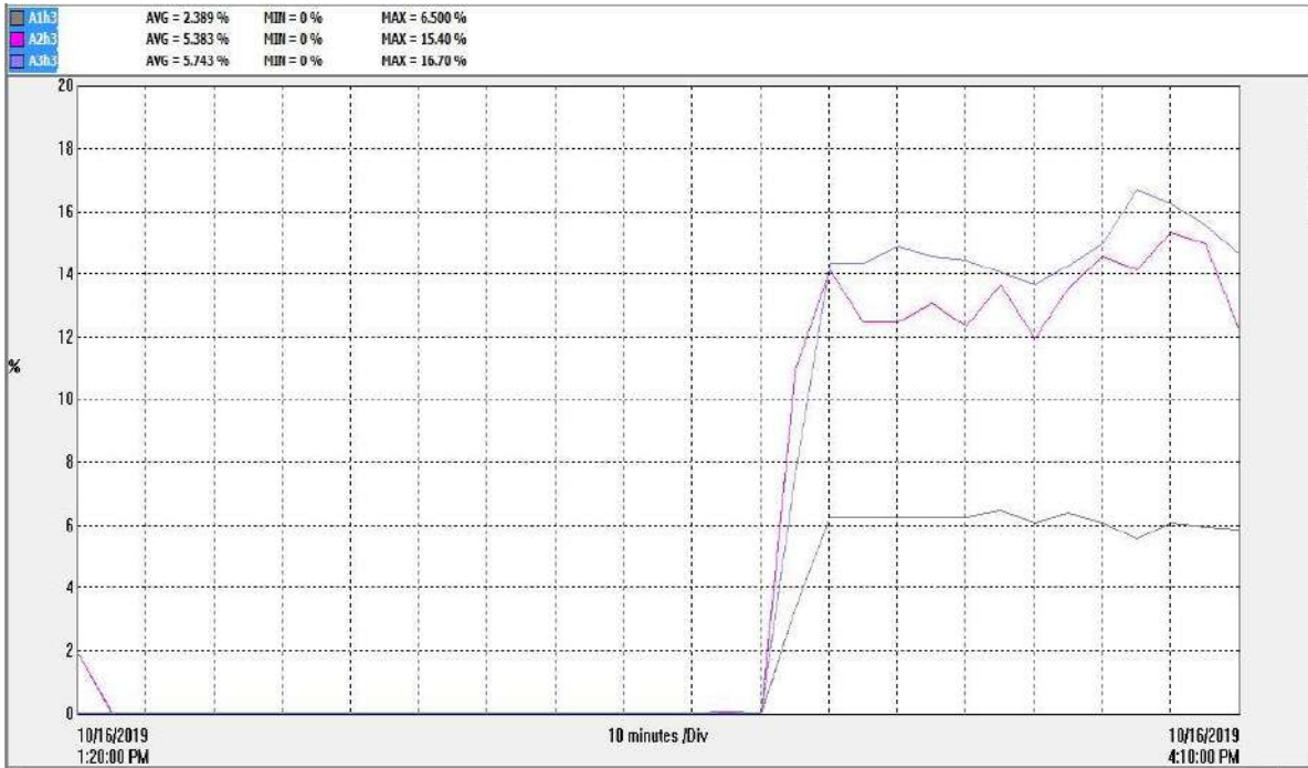
Fig.147 Shows the 3 th order THD (voltage harmonics) for 3.10 hours from 16/10/8/2019 12.00PM to 16/10/2019 4.10PM
