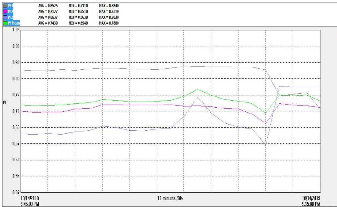
Fig.85 Shows the power factor (PF) for 2.0 hours from 14/10/2019 3.45PM to 14/10/2019 5.35PM Inference: No unbalanced found here. Need to be improve the PF.
