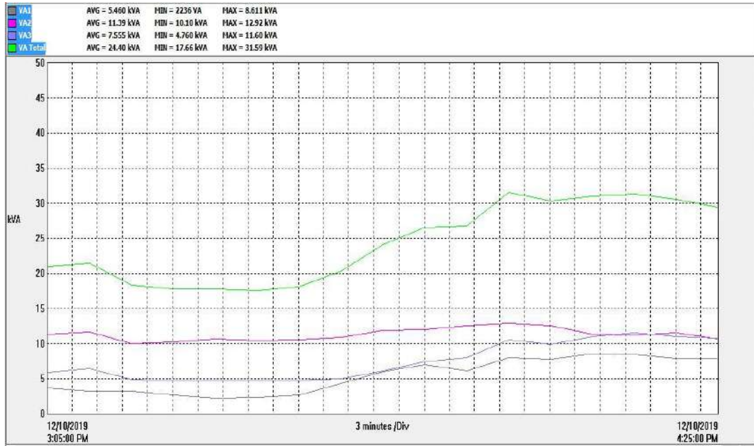
Fig 183. Shows the power (kVA) for 20MINUTES from 10/12/2019 12.55PM to 10/12/2019 4.25PM Inference: Phase 1 shows very low KVA.
