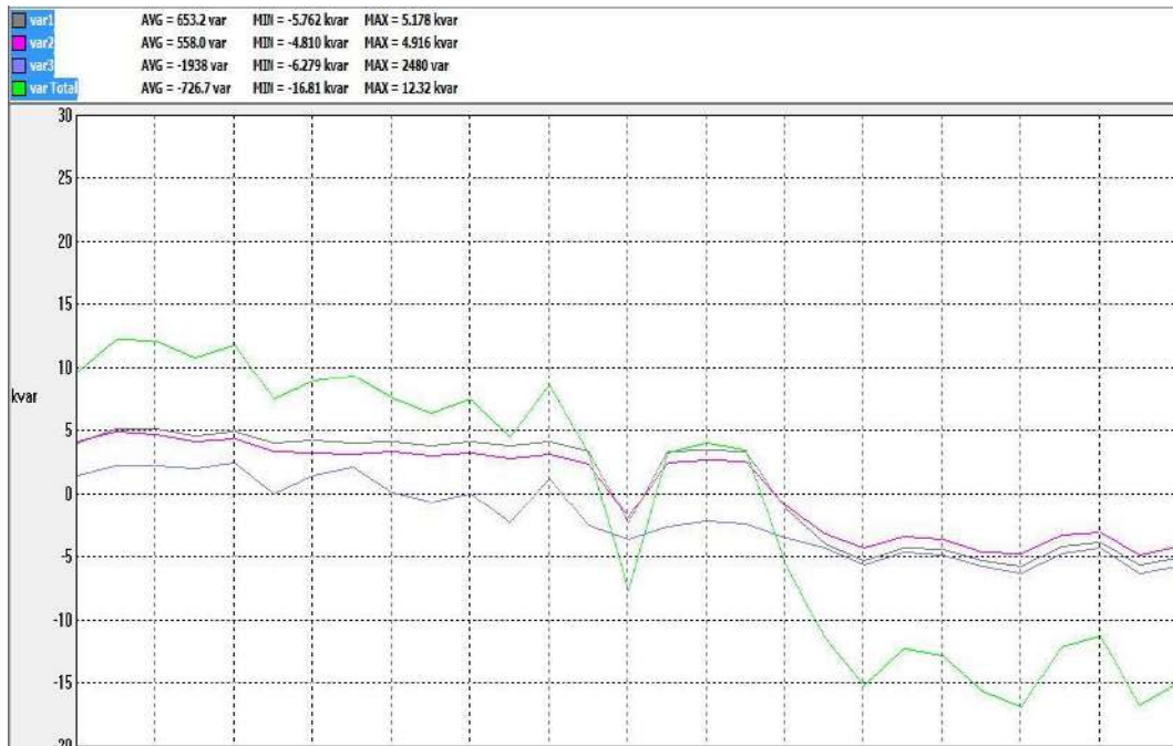
Fig.62 Shows the reactive power (kVAR) for 4 hours from 8/8/2019 5.00PM to 9/8/2019 4.20PM Inference: Phase 3 shows very low KVAR compare to other two phases. Need to be check.
